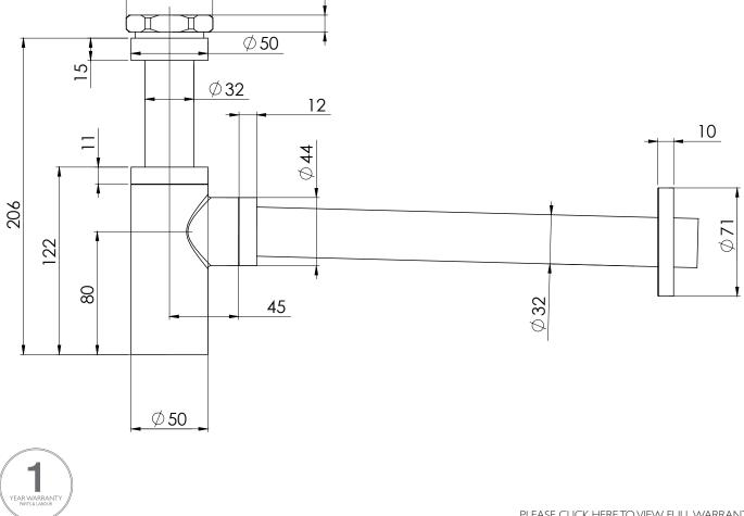
While we aim to ensure the specifications shown are correct at time of printing, Phoenix Tapware reserves the right to make modifications without prior notice. Always use the physical product measurements for mark-ups and roughing-in as the line drawing shown may differ from the actual product over time. All measurements are shown in millimetres.
