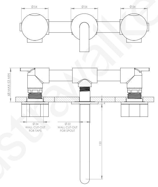
**NOTE**: Seat of Breech Body extensions are NOT recommended in conjunction with this Tapware. Failure to adhere will void warranty.
