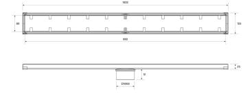
NOTE: Drains take tile thickness of 10mm
